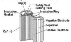
Never disassemble TENERGY batteries. Doing so may cause an internal or external short circuit or result in exposed material of battery reacting chemically with the air. It may also cause heat generation, explosion and fire. Also, this is dangerous as it may cause splashing of alkaline fluid.
