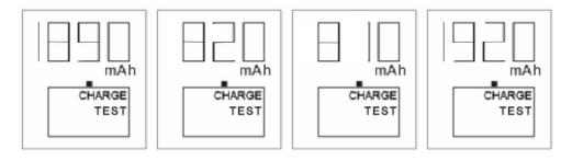
Stage 4 The testing process is over, trickle charge begins.
