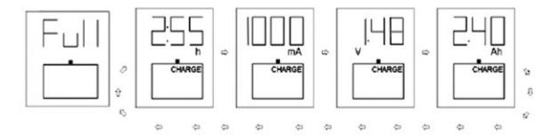
**Refresh Mode:** With the Refresh Mode, the battery is charged and discharged repeatedly to optimize to its maximum capacity. Old rechargeable batteries that have not been used for a long period of time can be restored to their rated capacity. Depends on the selected charge current, it can take hours or even days before completion.
