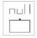
If batteries that are damaged or defective are inserted into the charger, the "null" icon will be displayed on the display and the charger will refuse to charge them.
