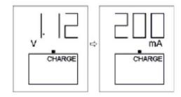
To change the charging current and/or operation mode, press and hold the Mode Select button for 1 second. After which the next available operation mode will be shown, and you can continue to press MODE to select other functions, or press CURRENT to change the charge/discharge current.
