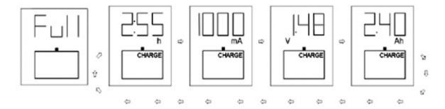
**Discharge Mode:** The Discharge Mode is used to reduce the memory effect. The rechargeable battery is discharged to a preset battery voltage (0.9V). Once a battery has been discharged, it will be charged at the pre-selected charging current. Discharging current is always half of the charging current.
