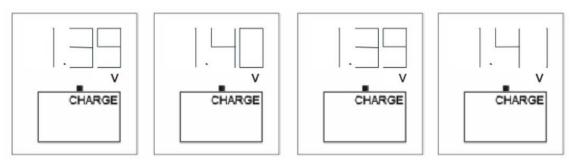
Stage3 Charge over, trickle charge.
