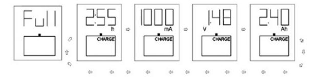
**Test Mode:** In Test Mode, the charger can measure a battery's capacity. The maximum capacity is determined by discharging the rechargeable battery after it has been fully charged. If the maximum capacity is much lower than the rated capacity, then it may have reached the end of its cycle life.
