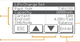
Li-Po/Li-ion/LiFe battery without PCB and/or requires balance charging must use Balance Mode with JST XH balancing connector. Always follow both the battery and charger instructions. Failure to do so may result in FIRE.
